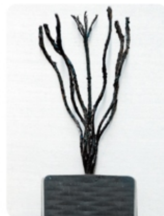
Good condition in penetrating of inner rubber
