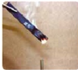
(2) Take the burner off, measure the flame duration time of the test specimen.
